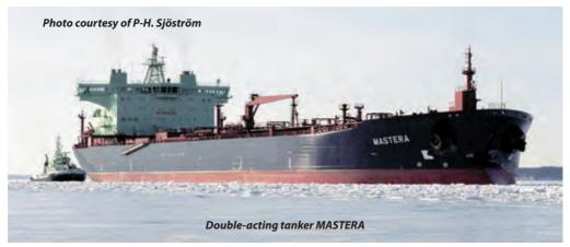
The principle of the DAT concept is that, like most vessels, it travels ahead on normal open water and thus has a highly hydrodynamic shaped bow and sides. When it sails in ice, however, it travels astern where the reinforced stern hullform is used to break the ice. The podded propulsion system is used to produce a water stream between the ice and the hull, thus lubricating the contact.
