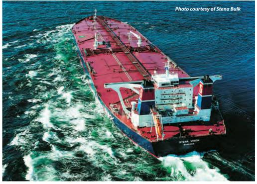
The aft-end of the vessel is characterised by the large transom stern, twin, widely-spaced funnels and an accommodation deckhouse which houses a complement of 34, plus 6 Suez crew and 4 repair men. Note the huge structure of the bridge wings.
