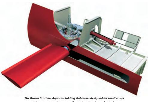
ships, passenger ferries, small naval and coastguard vessels. Fin area: 1.82 - 5.78 m<sup>2</sup>, total weight: 19.3 - 40.2 tonnes.
