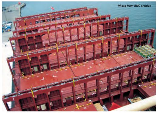
Lashing bridges on an ultra large container vessel
