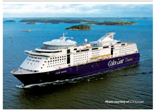
The ship is classified according to two all-new maritime standards: Det Norske Veritas Clean Class, defining environment-friendly design, as well as the Comfort Class, which secures a noiseless and vibration-free environment for passengers.
