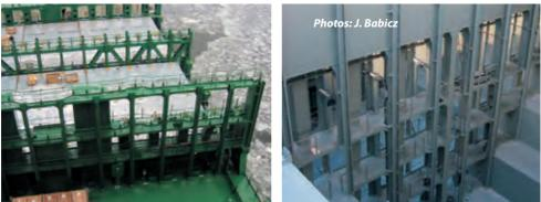
**Container cell guides** – Containers are commonly stowed below deck and sometimes on deck within fixed vertical cell guides, which guide them into place and ensure that they do not move during the voyage.
