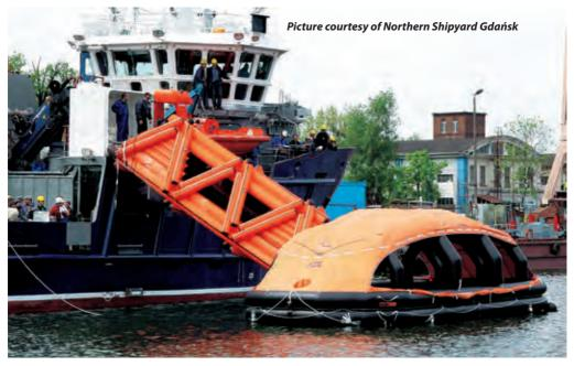
seconds of deployment, with the capability of evacuating 430 persons for each station well within the 30-minute timescale allowed.
