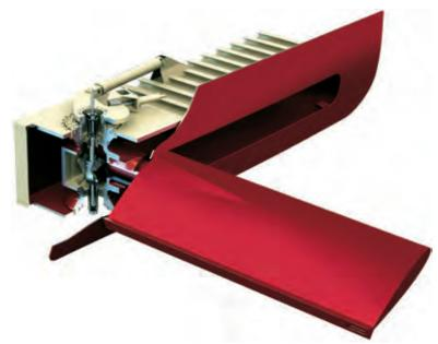
The Brown Brothers Neptun II folding stabilisers for large vessels. Fin area: 4.2 - 22.33 m<sup>2</sup>, total weight: 36.5 - 190 tonnes. The transatlantic liner QUEEN MARY 2 features four sets of 15.63 m<sup>2</sup> Neptune folding stabilisers.
