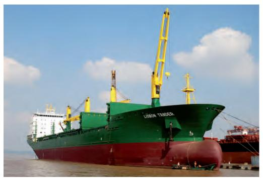
The hydraulically folded hatch covers are some of the heaviest which MacGREGOR has ever applied, since each of the seven bigger folding pairs weights appr. 140t. Two independent power packs are installed, supplied by two pumps each, serving up to 2 folding hatch cover pairs. The hatch covers have a breadth of 26.6m and form a 120m long continuous stowage plane, just interrupted by the crane columns and ventilation towers.
