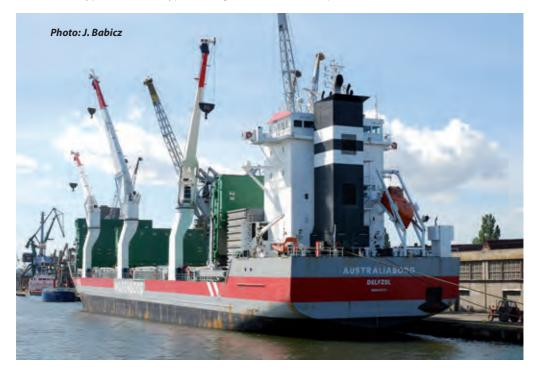
**Multi-purpose cargo ship** – The vessel designed for transport of wide range of commodities such as general cargo, forest products, dry bulk, grain, steel coils and usually equipped for transport of containers. Such vessels have tank top strengthened for heavy cargo and grab operation. Permissible tank top loading 10-20t/sqm.
