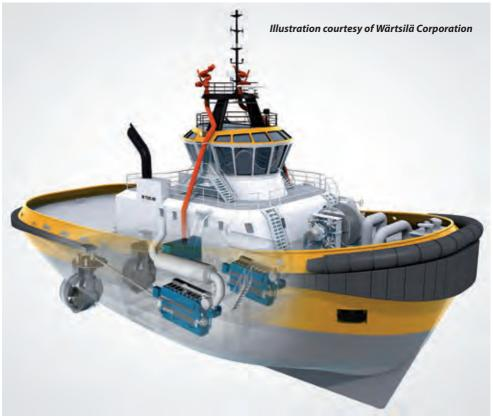
Escort tug W TUG 80 designed by Wärtsilä bollard pull 80 tonnes, speed abt. 14 knots, L<sub>OA</sub> 35.40m
