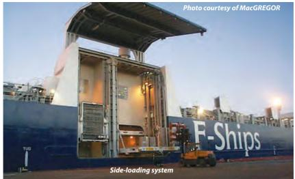
The cargo elevators connected to the loading platforms are designed to handle a paper reel load up to 16 tonnes with a maximum lifting speed of around 27m/min.
