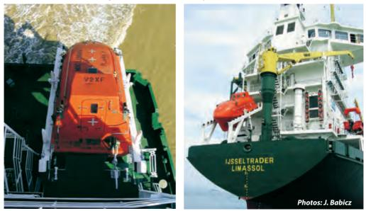
Free-fall lifeboat and simple launching ramp. Recovery by a combined life-saving/provisions crane
