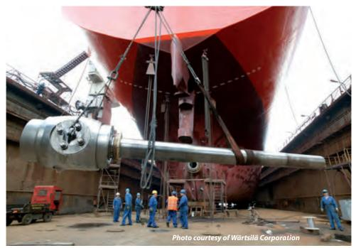
Propeller shaft with CP hub
