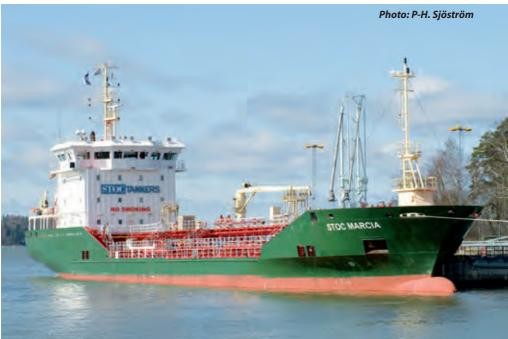
4634dwt oil/chemical tanker STOC MARCIA $L_{BP} = 94.04m, B_{mld} = 15.00m, D_{mld} = 7.40m, d = 6.00m$
