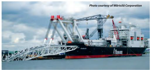
Dynamically positioned pipelying ship AUDACIA with the stinger on the bow. The stinger is made out of several hinged sections to make it articulated. Hence, the stinger shape and curvature can be controlled by setting these segments at chosen angles
