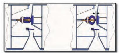
Omega seal secures weathertightness without air pressure in the inside air hoses
