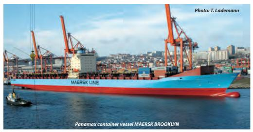
One two-stroke diesel engine Wärtsilä 12RTA96C, 68,640kW at 102 rpm, six-bladed FP propeller of 8555mm diameter.
