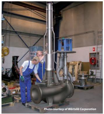
Deepwell cargo pumps offer a number of improvements, including the elimination of the traditional pumproom, greater pumping and stripping efficiency, more flexible cargo segregation, and corrosion-resistant stainless steel component construction.
