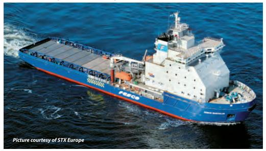
Its principal tasks will be to provide an all-year-round safety cover for the drilling platforms on the Sakhalin shelf, as well as transportat of dry, liquid and chemical cargoes. The vessel is also able to deal with oil spills and is equipped with a full outfit of skimming and collecting equipment. Operations will be aided by aluminium **workboat** which is lowered into the water by Dreggen crane.
