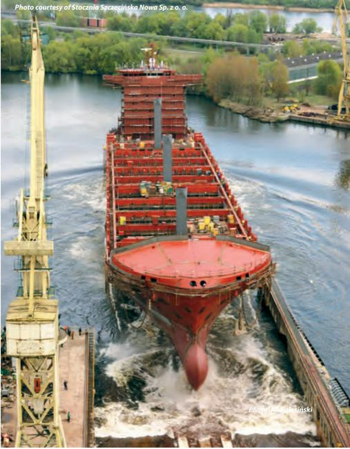
in a **dry dock**, floating off or **float out** is the equivalent of launching. **Ship elevator** and transfer system can be used to launch a vessel.
