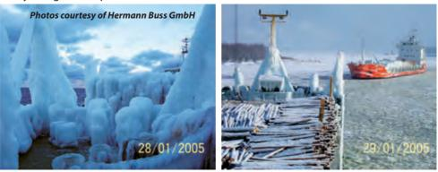
Ice accumulation can completely disrupt the functioning of certain deck equipment. The typical icing problems to be encountered are the impairment of stability due to the lifted center of gravity, limitation of safe navigation caused by antennae and radar equipment being out of operation and icing on **wheelhouse** windows.
