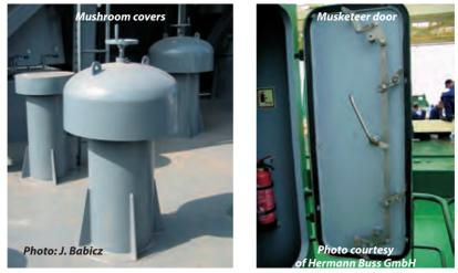
**Musketeer door** – Marine door with a novel locking mechanism developed by WINEL Company (the Netherlands). The Musketeer locking system incorporates a 33:1 power transmission from manual operating force to the locking device; as a result the door can be securely locked and opened even using an elbow or a shoulder only.
