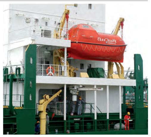
It is very important to arrange a good access to the lifeboat. Choose a davit which allow direct access without any boarding ladder
