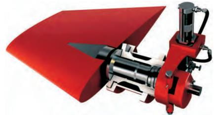
The Brown Brothers Gemini non-retractable stabilisers designed for smaller vessels. Fin area: 1.4 - 3.2 m<sup>2</sup>, total weight: 1.92 - 6.75 tonnes.
