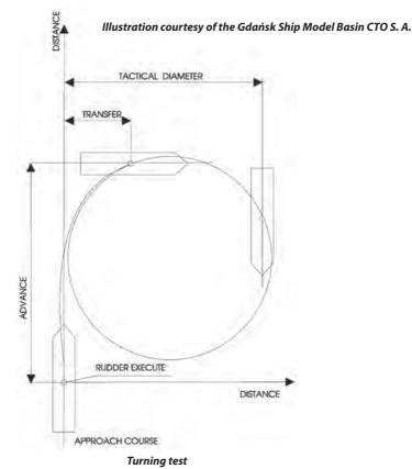
**Pull-out manoeuvre** – After a turning circle with steady rate of turn the rudder is returned to midship. If the ship is yaw stable, the rate of turn will decay to zero for turns both port and starboard. If the ship is yaw unstable, the rate of turn will reduce to some residual rate of turn. The pull-out manoeuvre is a simple test to give a quick indication of a ship yaw stability, however requires very calm weather.
