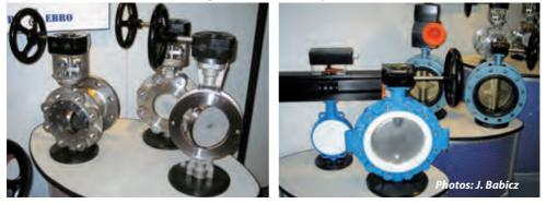
**Butterfly valve** – A rotary stem valve with a centrally-hinged disc of the same diameter as the pipeline. The valve opens into the pipeline and therefore takes up little space, permits large flow rates and gives minimum pressure drop.
