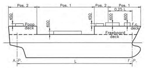
International Convention on Load Lines; Required coaming heights (mm) of hatches
