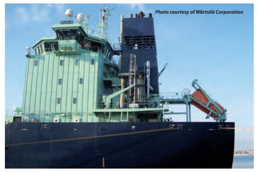
Test installation mounted in 2007 onboard a tanker MT SUULA  $SO_x$  reduction > 99%,  $NO_x$  reduction 5 –11%, PM reduction 30 – 60%
