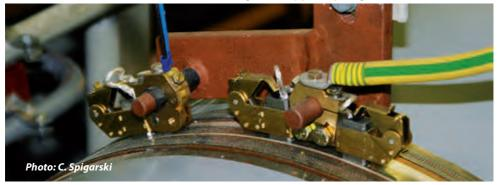
Shaft earthing device Figure courtesy of Wärtsilä Corporation 6 5 m Œ Propeller shaft 75 1. Silver/copper slipring Stainless steel badclamp
