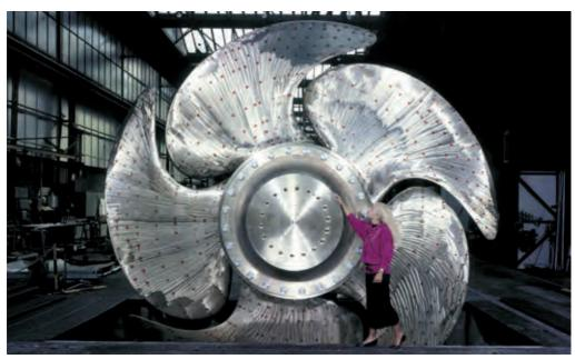
The world's most powerful CP propeller, installed on the Queen Elizabeth 2, 44 MW at 144 rpm, the propeller diameter is 6m, the hub diameter 2.0m
