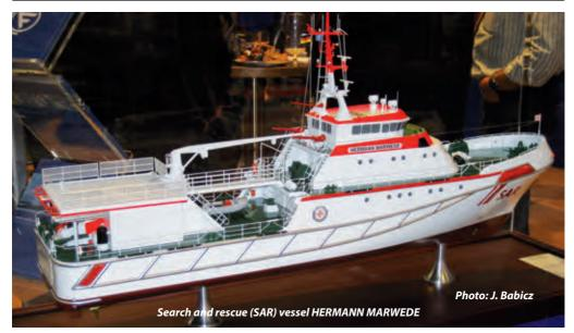
was delivered in 2003. With a length of 45.6m, a beam of 10.6m and displacement of 400 tonnes, this new rescue cruiser is the largest in DGzRS fleet. There are two engine rooms, with two 2040kW MTU 12V 4000 M90 wing engines in the forward compartment and a 2720kW 16V 4000 M90 centreline diesel aft. Each of the three engines drives a fixed pitch propeller through Reintjes gearing.
