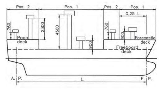
International Convention on Load Lines; Required ventilator coaming heights (mm)
