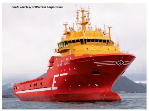
The first gas-fuelled PSV VIKING ENERGY In ten years of operation not a single hour of technical offhire has been caused by the gas system
