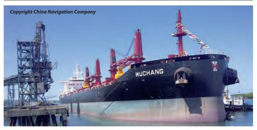
Handymax bulk carrier WUCHANG of B.Delta 37 type designed by Deltamarin The vessel is fitted with a low-speed Wärtsilä 5RT Flex 50-B engine that has a power 6060kW, which gives the vessel a service speed of 14 knots.
