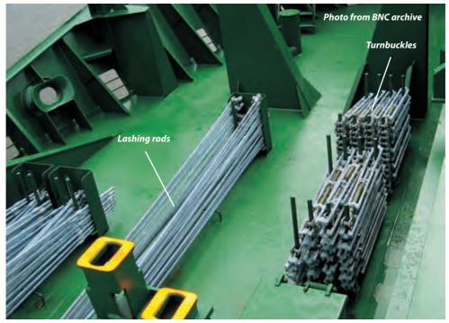
Stowage of lashing rods and turnbuckles
