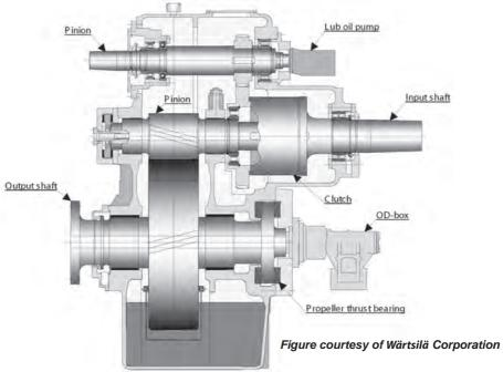
Cross-section of the single stage single input gear with clutch and primary PTO
