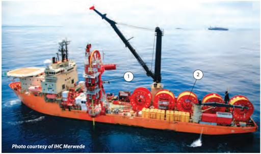
Multi-purpose offshore vessel TOISA PERSEUS 1. Vertical lay tower 2. Storage reel
