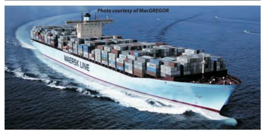
ESTELLE MAERSK 15,500 TEU Maersk Line PS-class mark the introduction into service of the first 14-cylinder RT-flex96C Wärtsilä engines developing 80,080kW
