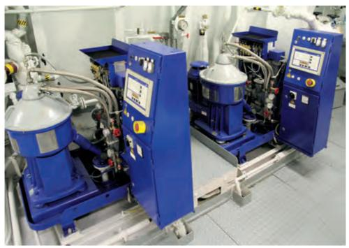
Separation system modules from Alfa-Laval
