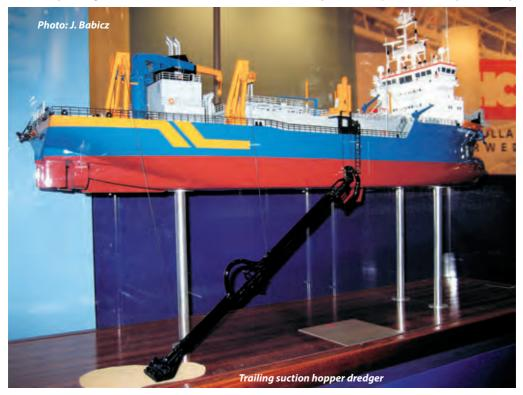
positioned; the dredger uses its propulsion equipment to proceed over the track. It is a shipshaped vessel with hopper type cargo holds to store the slurry. At each side of the ship is a suction arm, which consists of a lower and a higher part, connected through cardanic joints. Trailing suction hopper dredgers are used for maintenance work (removal of deposits in approach channels) and dredging of trenches in softer soils.
