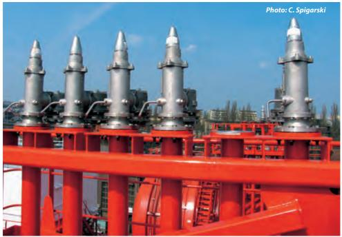
Pressure-vacuum valves on a chemical tanker
