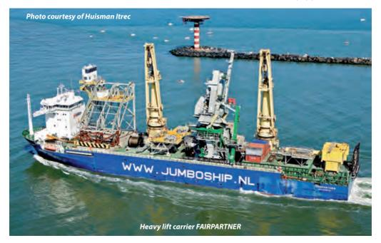
additional hoists: a sling handling hoist (SWL10t), an auxiliary hoist (SWL37.5t) and a tugger hoist (SWL25t, 200m length). Both cranes are controlled by a small portable and wireless control panel, which allows control from anywhere on the vessel or even from the quayside. When the wireless signal from the control unit is interrupted, the crane automatically stops any activity and hold its position.
