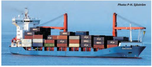
Feeder vessel: note the enclosed bridge
