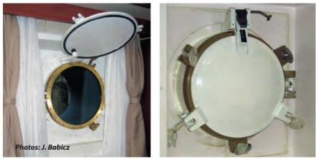
Sidescuttles are divided into three types: Type A (Heavy), type B (Medium) and type C (Light). The minimum requirement for type A is that it shall withstand a water pressure
