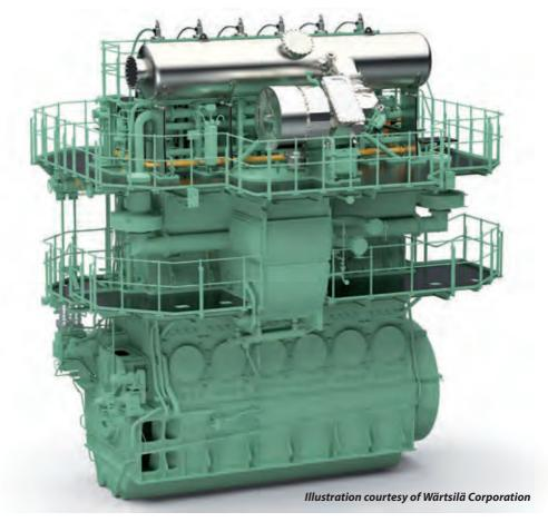
Low-speed low-pressure dual-fuel engine RT-flex 50DF meets IMO Tier III requirements without exhaust gas after-treatment due to lean burn Otto combustion process
