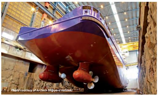
A double acting ship, VITUS BERING is designed to be able to break ice both ahead and astern
