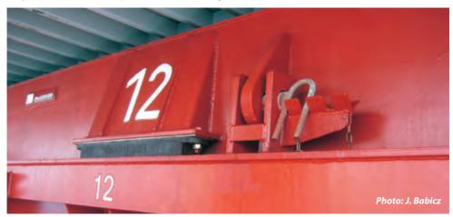
Fixpad – Welded steel pad with the mating surface of wear-resistant steel.
