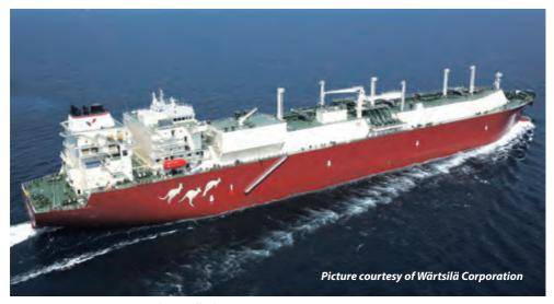
*Electrically driven LNG carrier WOODSIDE ROGERS* The four central tanks has a total capacity of 159,760m<sup>3</sup>. The electric drive system is supported by four tri-fuel Wärtsilä 9L50DF engines, which are installed in two separate engine rooms.
