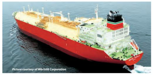
The 39,900kW power plant is based on four dual-fuel Wärtsilä 50DF engines. Two 12-cylinder vee-type DF engines, rated at 11,400kW, and two with nine cylinders in line models, producing 8550kW apiece, drive four Converteam generators. The four-engine arrangement and distribution of machinery in two separate engine rooms confers a high degree of redundancy.
