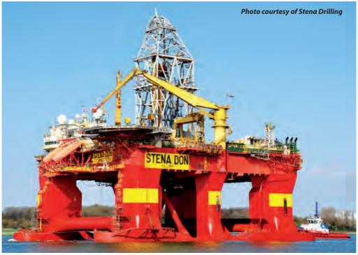
Semi-submersible drilling unit
