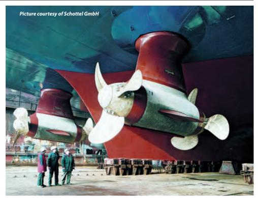
connected to the pod. This means that the heat generated in the motor is conducted to the surrounding water without any need for internal air or water cooling system.
