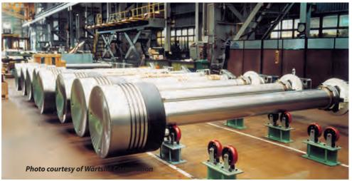
**Piston** – A cylindrical metal item which reciprocates within a cylinder. It may move as a result of fluid pressure as in an engine, or it can compress a fluid, as in a pump or compressor. The piston consists of **piston crown** and **piston skirt** screwed together.
