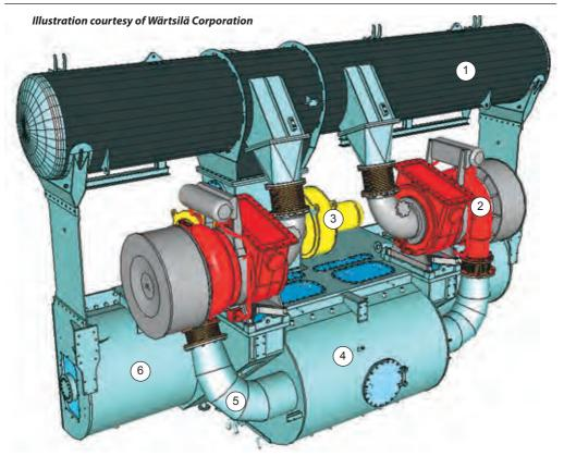
Complete scavenging system for Wärtsilä SULZER RT-flex60C engine, comprising exhaust manifold "1", two turbochargers "2", axiliary blowers "3", scavenge air cooler "4", scavenge air pipes "5", and scavenge air receiver "6"
