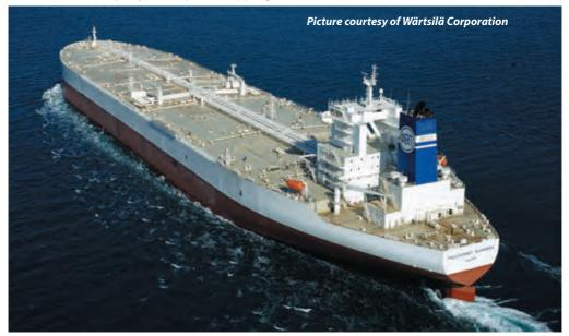
Nicknamed the "white elephant" because of its appearance of a wide-bodied white hull, the HELLESPONT ALHAMBRA is the first ship in a four-ship contract placed with the South Korean shipbuilder Daewoo Shipbuilding & Machine Engineering Co. The ship is the largest double hull tanker ever built and is reported to have cost about \$90 million. The design for these high specification of 3.2 million barrel vessels was subject to extensive model tests
