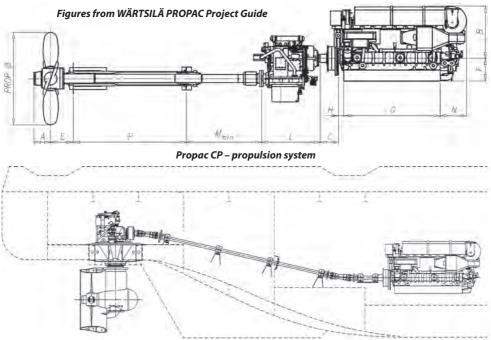
Propac ST – arrangement with fixed propeller thrusters, cardan shafts and slipping clutch
