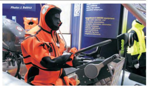
when boarding fully enclosed lifeboat. The experience gained after the January 2007 abandonment of the containership MSC NAPOLI shown the potential risks resulting from wearing immersion suits in fully enclosed lifeboat. Although outside temperatures were frigid, the members of the crew who wore immersion suits suffered from overheating and dehydration.
