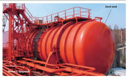
Gravity tank - A cargo tank with design pressure not exceeding 0.7 bar gauge.
