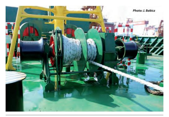
**Three speed pole-change drive** – The nearly maintenance-free electric motor is equipped with standstill heating, temperature sensors and fail-safe brake. The winch control is precise and easy. Speed steps in both directions are obtained by a single lever. Electric systems are easy to install and provide quick start in all environmental conditions.
