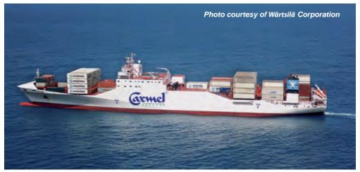
An interesting feature is the adoption of an innovative arrangement with the **superstructure** located amdiships above the large, fully-insulated refrigerated hold. Three conventional cellular holds are placed forward of this hold and two aft, offering places for 266TEU. Additional 630TEU can be carried on hatch covers and open deck provided with **lashing bridges**.
