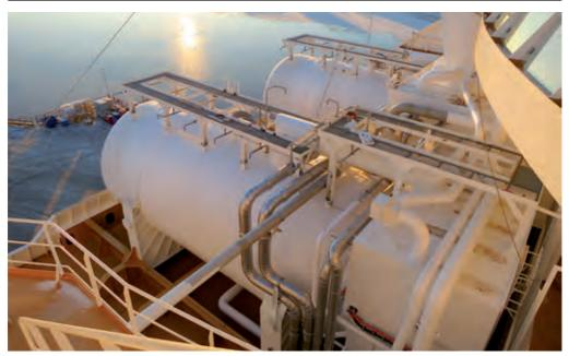
Wärtsilä's patented Cold Recovery System utilises the latent heat of LNG in air conditioning systems, reducing the amount of electricity consumed in cooling compressors. Significant operational savings and an increase in overall vessel efficiency are the result.
