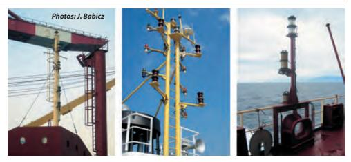
Navigation lights – All seagoing ships must be equipped with running and signal lights in compliance with the International Regulations for Preventing Collision at Sea (COLREG). A navigational light panel is installed in the wheelhouse for the control of all running and signal lights.
