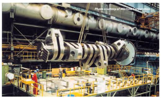
Fitting the crankshaft into the bedplate
