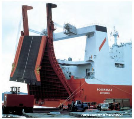
Ro-ro vessels berthing at quays with considerable height differences require long ramps. To avoid stovage problem, foldable stern ramps can be used. The foldable stern ramp/ door comprises two main sections articulated together and provided with outer and inner flaps to allow smooth transition of vehicles. When in the closed position, the inner section acts as a weathertight door, secured by hydraulically-operated cleats and locking devices.
