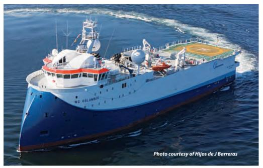
WG COLUBMUS – first seismic ship with Ulstein's X-Bow LOA = 88.8m, Bmld = 19.0m, D = 8.0m, 69 berths
