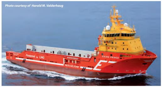
The general layout of PSVs has become fairly standardized, with a large open working deck aft and the accommodation forward. They have low angle of deck immersion due to small depth in way of open working deck
