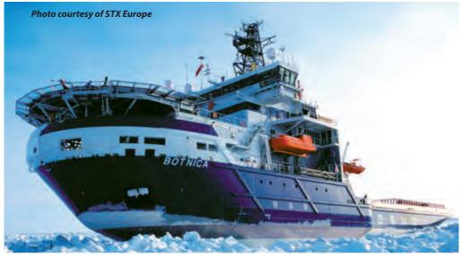
The new vessel is somewhat smaller than its predecessors. FENNICA and NORDICA were 116m long with a beam of 26m and 15 megawatts of propulsion power, fed through two azimuth **thrusters**. BOTNICA is 96.7m long with a 24m-beam. The total engine output is15MW but under normal conditions 10MW is used for propulsion. The latest technology has been incorporated and BOTNICA is notable for two **Azipod** units which provide a **bollard pull**
