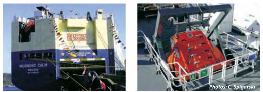
Free-fall lifeboat and launching ramp with integral recovery system onboard car carrier
