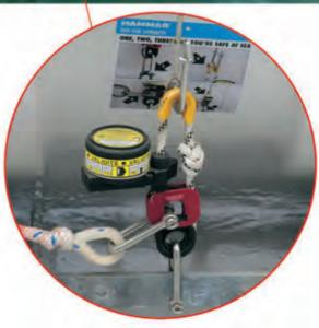
Hydrostatic release unit (HRU)
