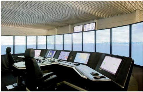
**Navigating and manoeuvring workstation** – The main **workstation** on the **bridge** where speed and course are considered and controlled, preferably conceived for working in the seated position with optimum visibility and integrated presentation of information and operating equipment. It shall be possible from this place to operate the ship safely, in particular when a fast sequence of action is required.
