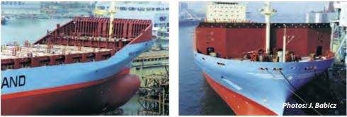
Standard breakwater on the 2200TEU container vessel
