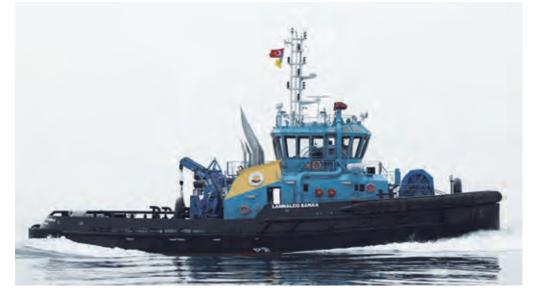
The principal particulars of this RAstar 3600 Class tug are: Length, OA: 35.80m, Beam, moulded: 14.50m, Depth, moluded: 6.03m (above design baseline), Maximum operating draft: 6.50m (to underside of drives), Bollard pull, ahead/astern: 118t/110t maximum, Free running speed, ahead: 15.1 knots, Lightship mass: 963t.
