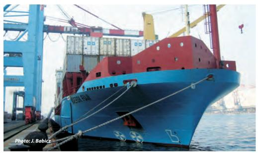
New type of the breakwater applied by Jan Babicz. Such breakwater protects not only cargo but windlasses and mooring winches as well
