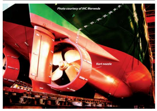
Kort nozzle – A fixed, annular forward extending duct around the propeller. The propeller operates with a small gap between blade tips and the nozzle internal wall, roughly at the narrowest point. The nozzle ring has a cross-section shaped as a hydrofoil.
