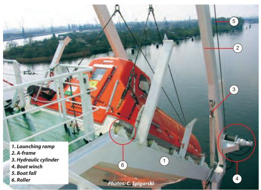
Launching ramp with the integral recovery system
