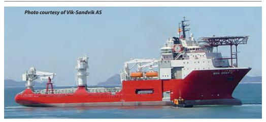
guide winches and powered guide pins also installed. BOA DEEP C also boasts twin built-in deepwater ROVs of Oceaneering Millenium type and a 7.2mx7.2m moonpool. The ROVs are located in hangars. Over the side a guided launching system for extreme condition operation is provided.
