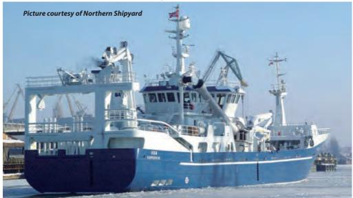
The ship designed by Sawicon AS VEA is capable of trawling and purse seining and measures 60.40m overall with a beam of 12.60m, and a depth of 8.10m. The steel hull is topped with an aluminium superstructure. The layout has the trawl handled over the stern, with arrangements for the content to be brought forward and pumped out over the starboard side, with the separator and access to the fish tanks on the forward deck. The purse seine is handled and hauled over the starboard side.
