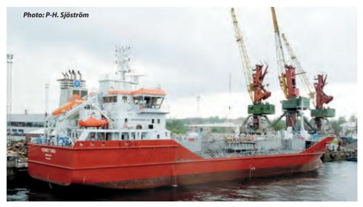
**3515dwt product carrier VEDREY TORA LBP = 75.00m, Bmld = 15.70m, Dmld = 7.80m** VEDREY TORA has the main engine Wärtsilä 6L26 running on gas oil, MCR = 2025kW, service speed 12.5 knots.
