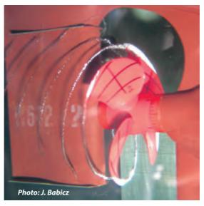
tested with the complete hull-propulsion appendage as an integrated unit, and tests are carried out at high Reynolds numbers, that is with high velocities.
