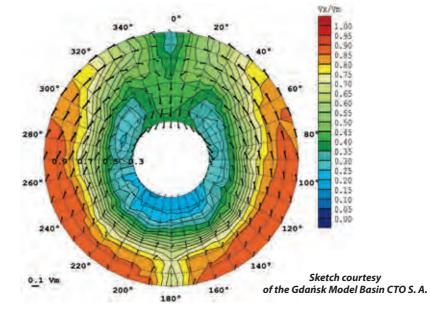
of the boundary layer increases with its distance from the bow. The layer is therefore the thickest at the end of the hull. It means that there will be a certain wake velocity caused by friction along the sides of the hull. Additionally, the displacement of water by the ship will also cause wake waves both fore and aft. All this results in the propeller behind the hull is working in non-uniform water flow called wake-field.
