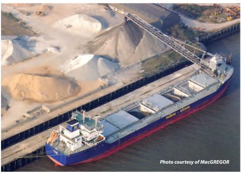
Gravity-type self unloader system on the 28,400dwt STONES
