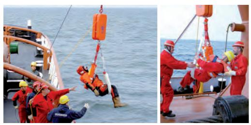
Rescue lifting system with double loop and stopper block
