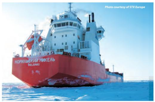
Double-acting container vessel NORILSKIY NICKEL
